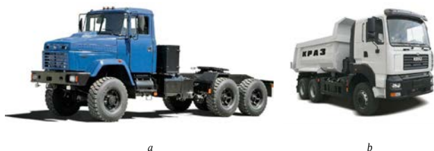
Fig. 1. Four-wheel drive vehicles: a – KrAZ-6446 Burlak truck tractor; b – KrAZ-6511C6 dump truck
